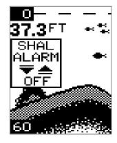
reaches the desired setting, release the arrow key. When the bottom depth goes shallower than the alarm's setting an alarm tone sounds. At the same
